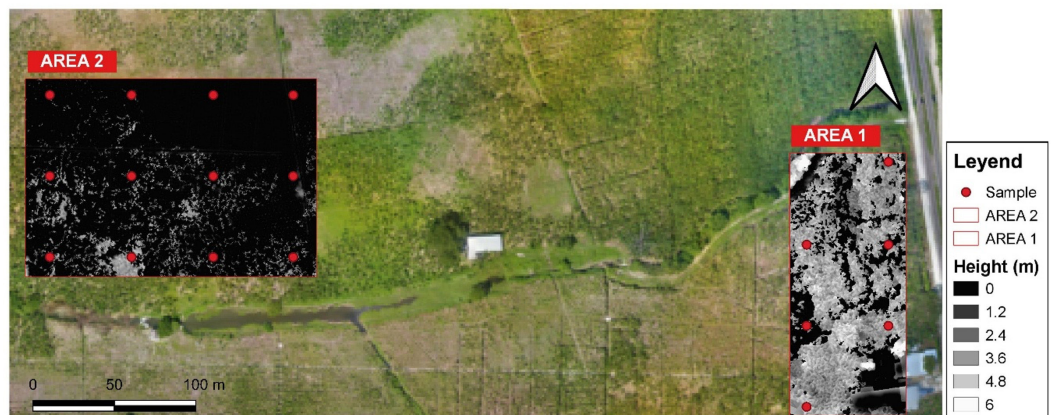
Figure 3: CHM derived from photogrammetric processing of RGB images.
